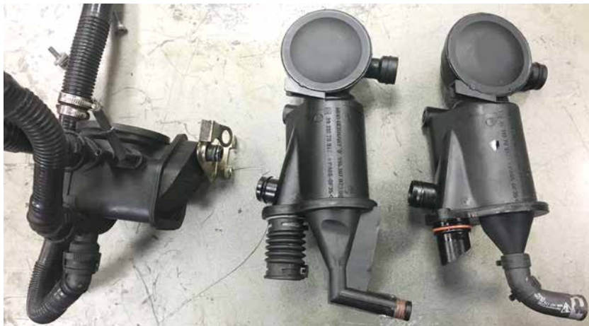
Air/oil separators — On the right is the 2002 up M96. In the center is the 1997-2000 Boxster. And on the left is the A/OS for the 2006 (and later) M97/O1.
