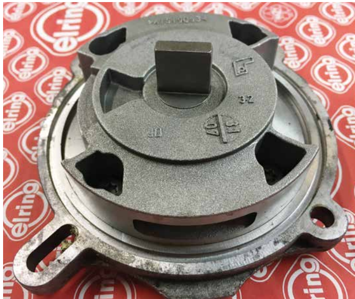
This shows the single stage M96 scavenge pump.
