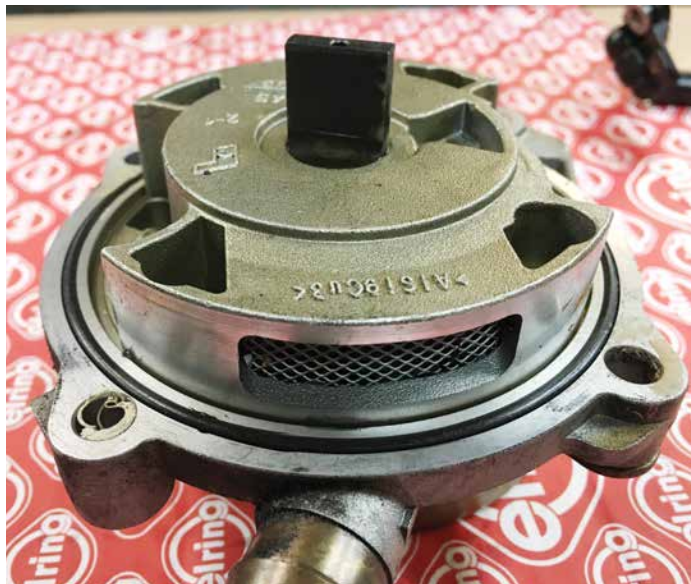
Inside drive for the tandem pump — note debris screen
