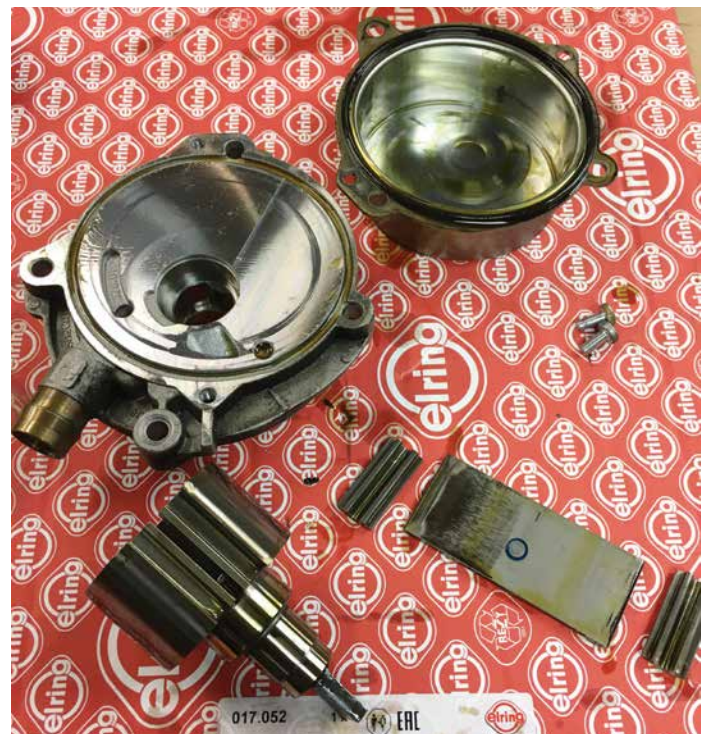
Here we have the tandem oil scavenge/vacuum pump. Note the vanes and seal plates at the vane apex.
