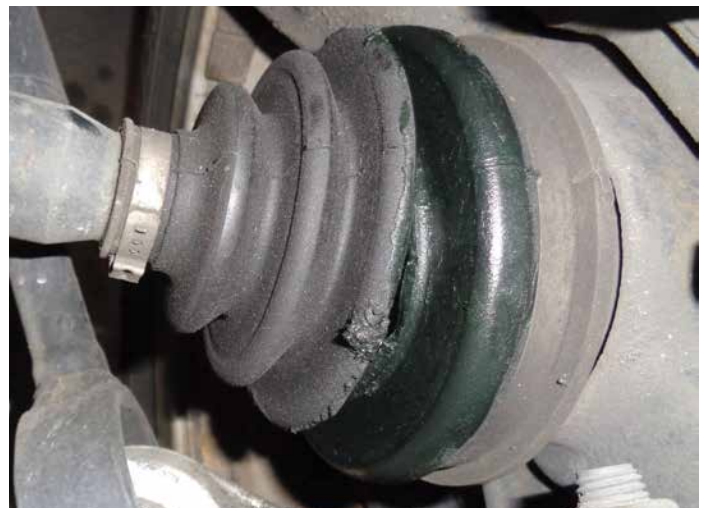
Dry rotting rubber in the gaiter is the most common cause for a C-V boot failure to occur.
