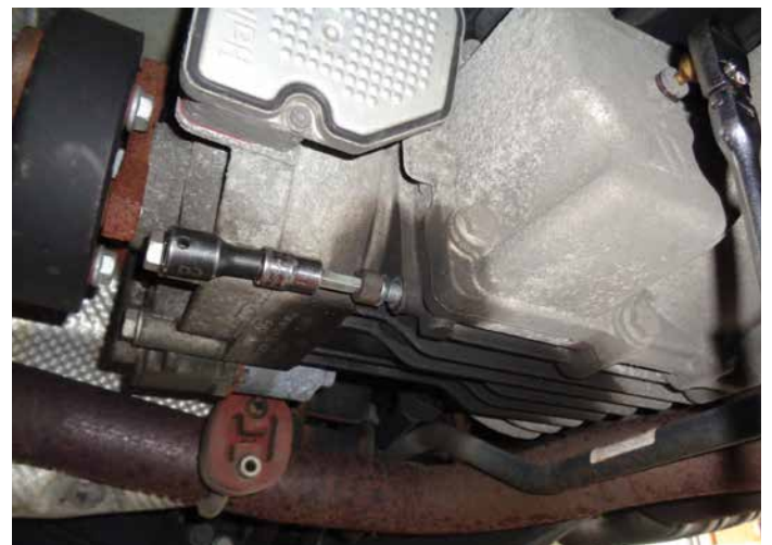
Don't confuse the rear differential drain with the easy-to-miss Haldex drain bolt.
