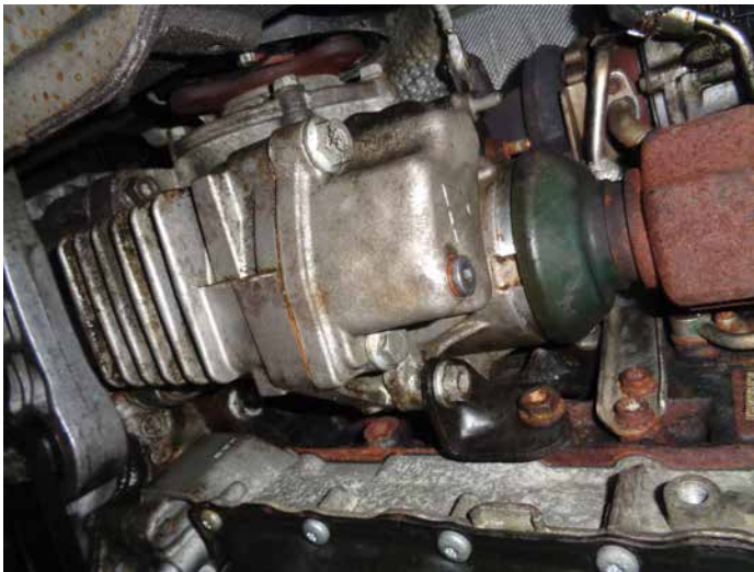
This is the front differential on an Audi A3 model. Note: It resides directly below the turbocharger.
