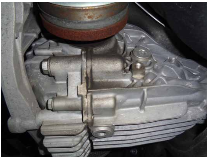
The drain and fill plugs are clearly visible on the passenger side of rear differential assembly.
