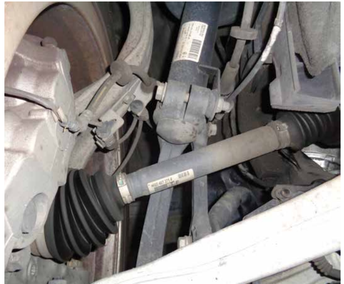
The front outer axle joint takes the most abuse out of all the driveline's components.
