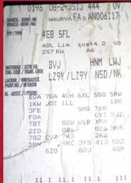
The ID tag is often worn or water damaged and may be difficult to read.
