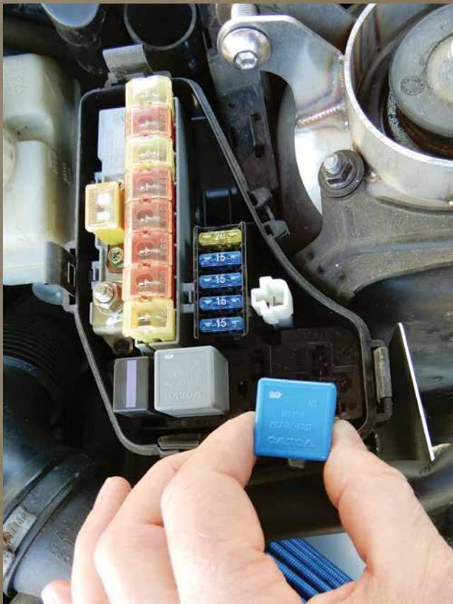
Fuse box main relay and B+ terminal
