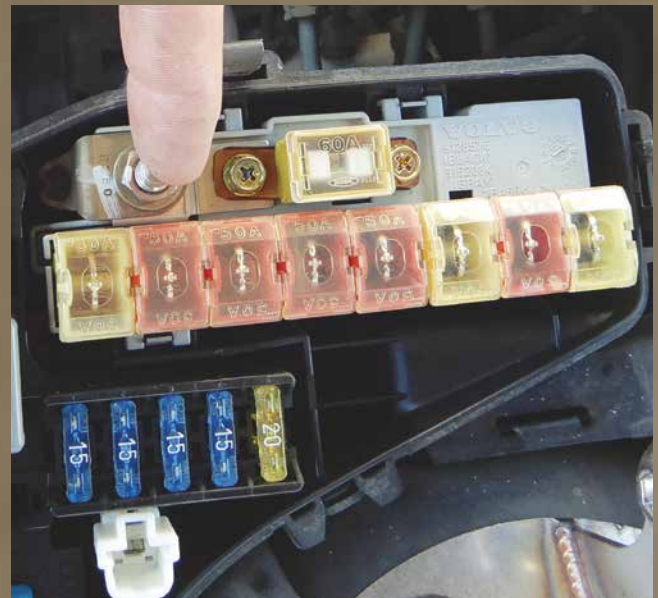
Harness connected at fuse box 13 mm nut
