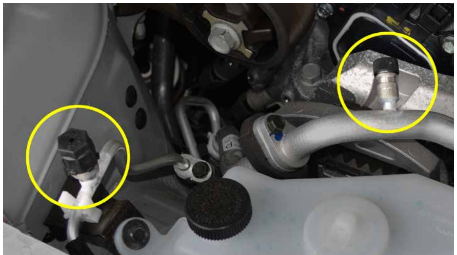
R-1234yf A/C systems have service ports and fittings of different size and shape to prevent cross-contamination with other refrigerants.
