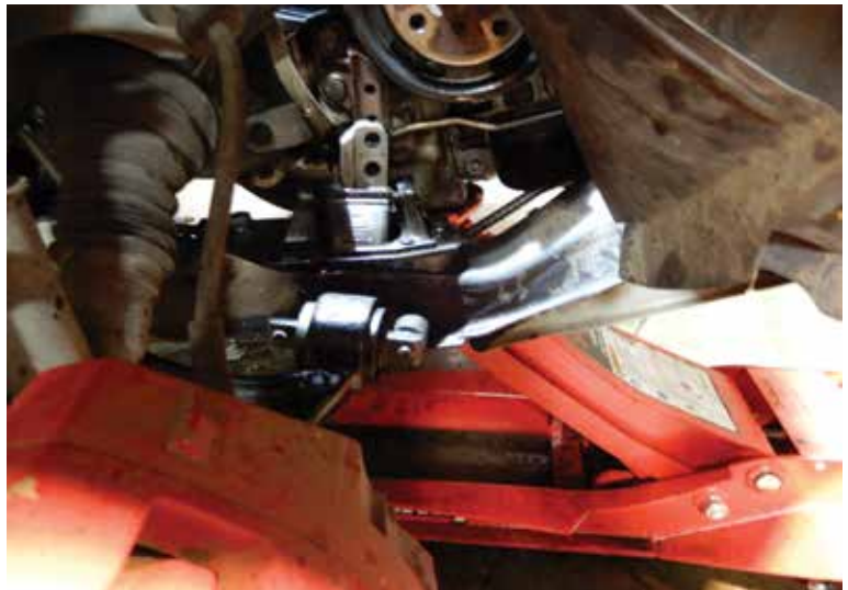
Jack under front of oil pan holding engine up
