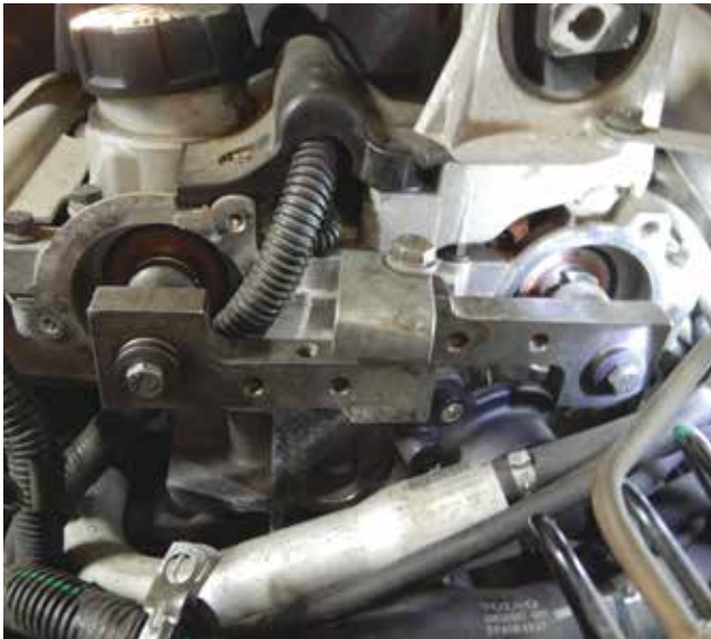
Tool installed on back on camshafts
