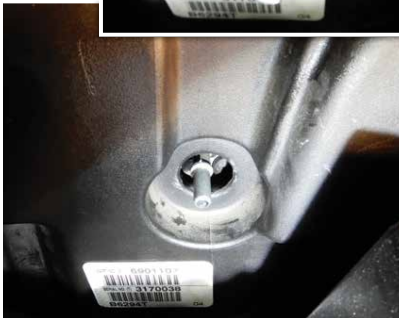
Front timing belt cover installed with the water pipe from the thermostat sticking through the cover
