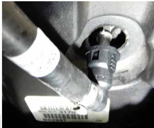
Front timing belt cover installed with the water pipe from the thermostat sticking through the cover
