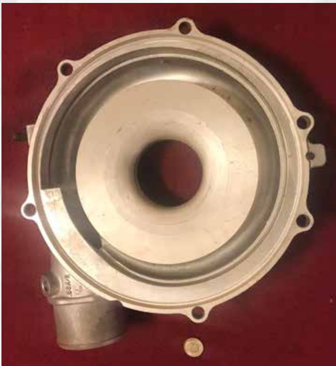
Bigger is better...sometimes. Can you imagine the amount of exhaust flow necessary to get this huge turbo to wind up? Ultimate horsepower comes at the expense of substantial turbo lag.
