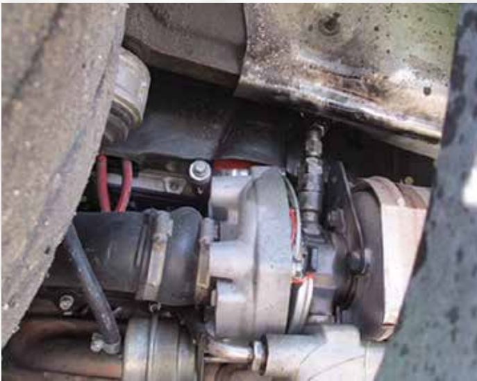
This turbo's impeller was lightened and balanced by someone lacking skills and equipment. The result was a total loss of the turbo itself. Note the pieces trying to escape from the housing.
