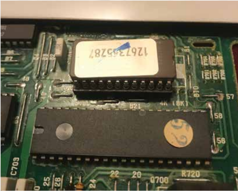
Replaceable and programmable EPROM sits in the brain and signals valves controlling the turbocharger.
