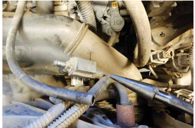
Smoke testing a vehicle
