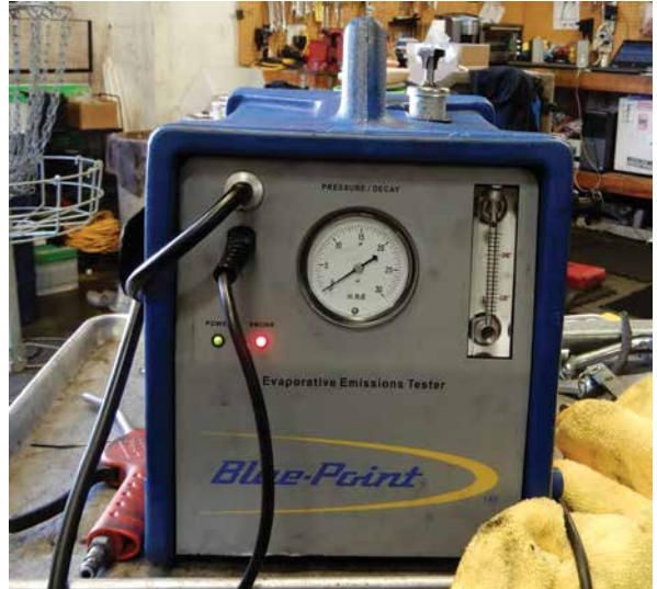
Smoke testing a vehicle
