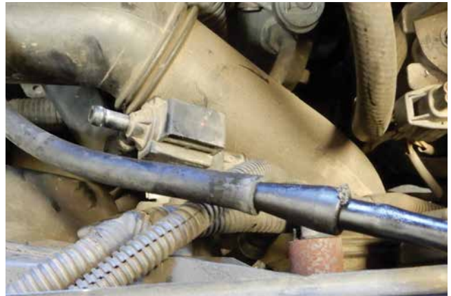
Smoke testing a vehicle and leaking hoses at the canister
