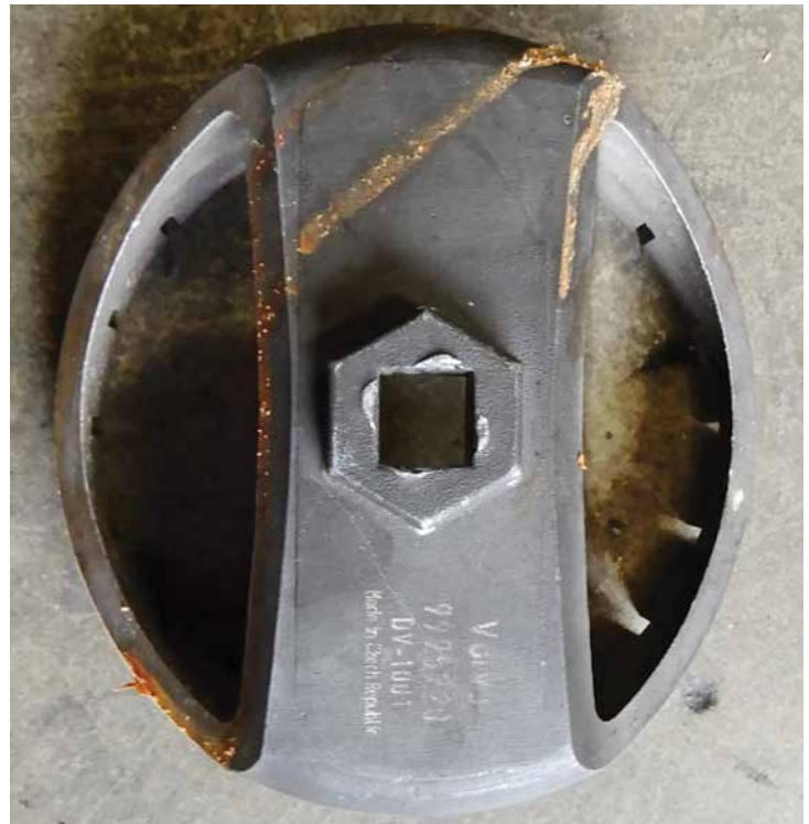
Using Volvo special tool number 9995720 to remove plastic collar
