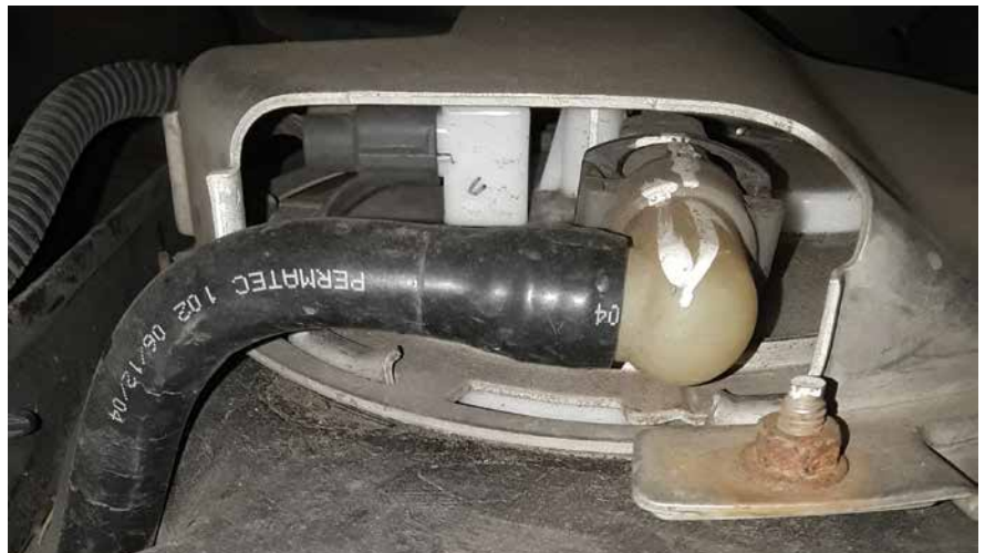
Having a tough time filling the tank? Disconnect this EVAP vent pipe and see if it fills easier. A blockage in the vent system will make re-fueling difficult as it will repeatedly trip the safety on the filling station pump handle.
