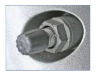
✓ This is the new black rubber tire valve/TPMS transmitter used beginning with 2008 models.
