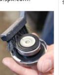
any remaining debris may result in continued coolant overflow loss. If there is an excessive amount of debris or the sealing rubber on the cap appears to be pitted or damaged, replace the cap.
