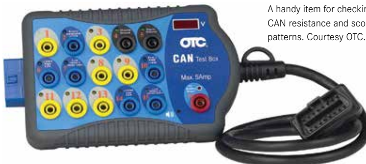
Note the labeling of the test leads making it easy to connect to your lab scope for diagnosis.
