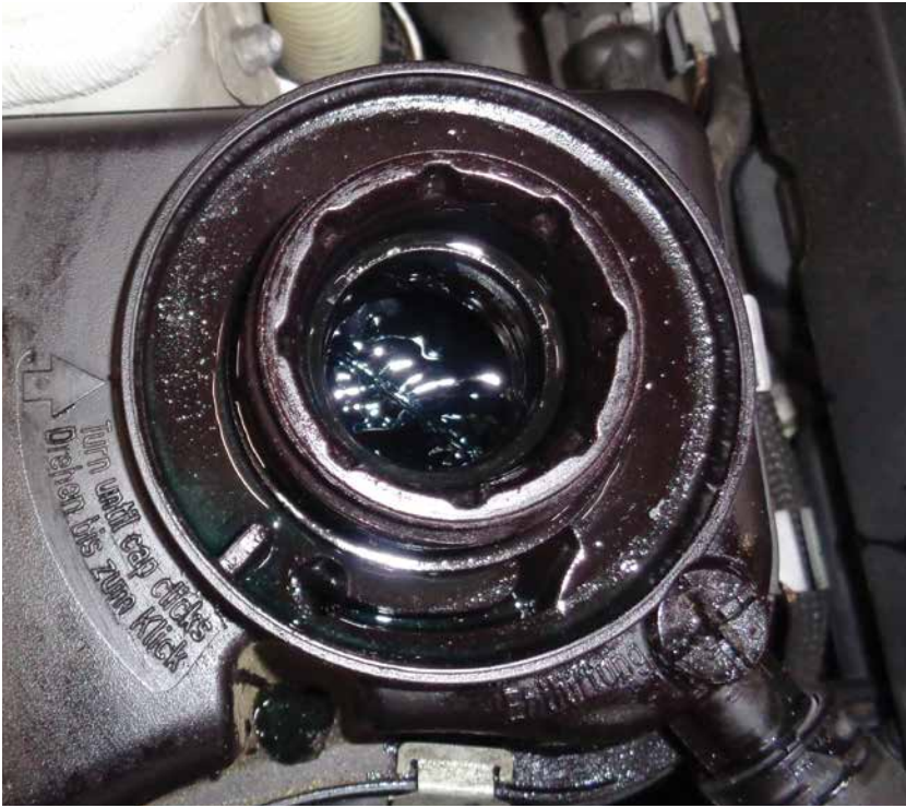
The coolant pump can be heard to run and coolant flow can be visible at the expansion tank during the process.
