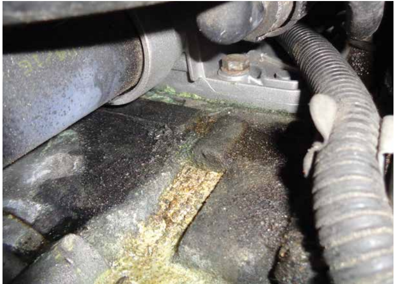
The valley pan is a notorious location for coolant leaks.
