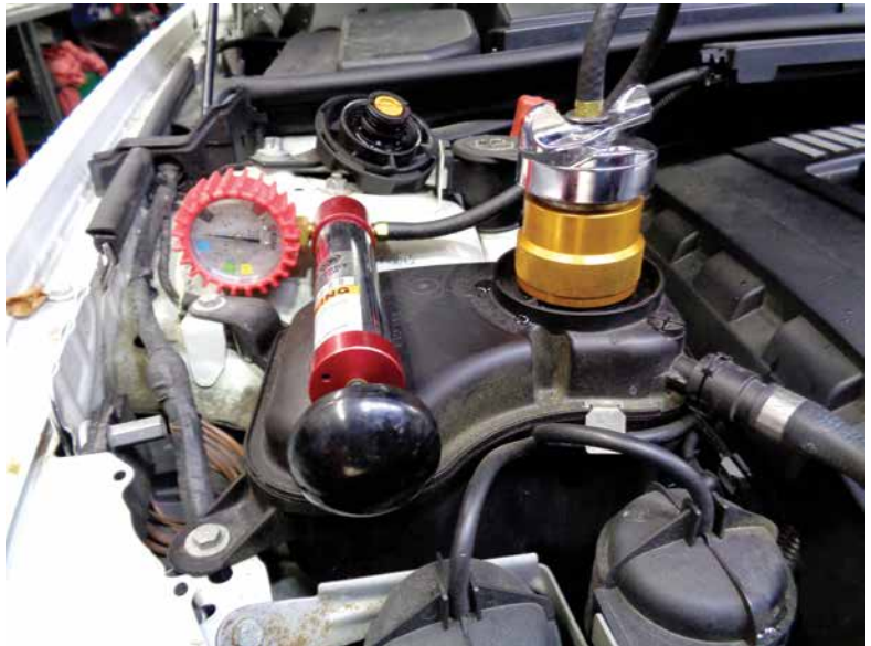
A reliable coolant pressure tester with BMW adapters is an absolute necessity when chasing down leaks.
