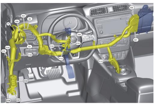
The Nissan Electronic Service Manual (ESM) shows a realistic "see-through" illustration of the 2019 LEAF e-Pedal system, making it easy to locate and identify key components. A separate table gives definitions of the numbered items in the callouts. E101 is the Accelerator Pedal Position Sensor, E112 is the Brake Pedal Position Switch, E36 is the Stroke Sensor, E72 and E104 are Body Grounds, and so forth.
