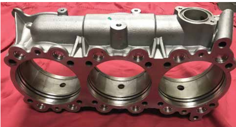
Picture of the housing where the water-cooled cylinder sleeve is housed
