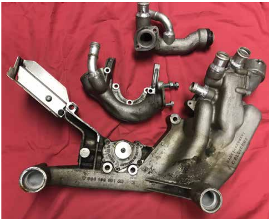
These are the external coolant manifolds for a 996 twin turbo Porsche engine.
