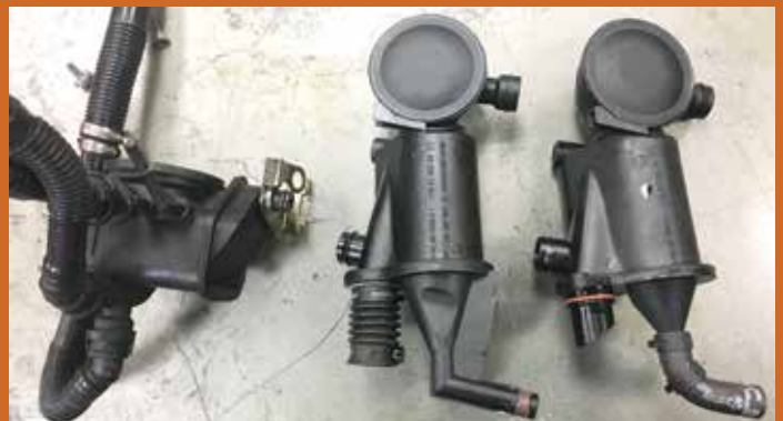
Air/oil separators — On the right is the 2002 up M96. In the center is the 1997-2000 Boxster. And on the left is the A/OS for the 2006 (and later) M97/01.
