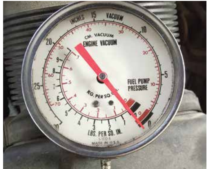
Correct vacuum - very little movement of the gauge at idle.
