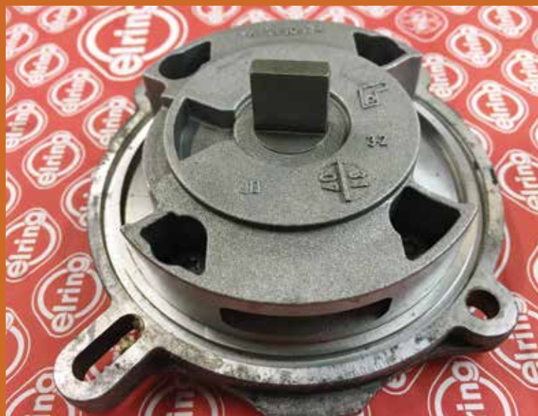
This shows the single stage M96 scavenge pump.
