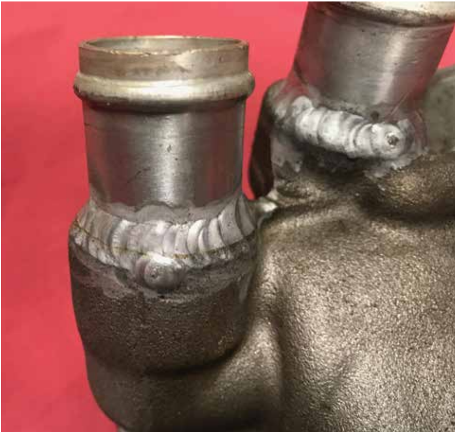
Example of a high-quality TIG welded connection of the coolant manifold to the flanged tube.
