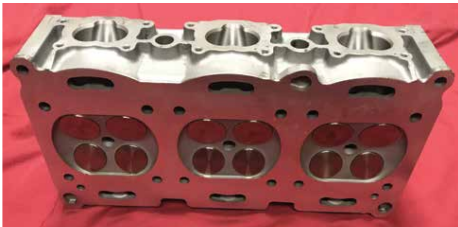
A cylinder head for a water-cooled Mezger engine. This is one piece, as opposed to individual heads on the air-cooled versions.
