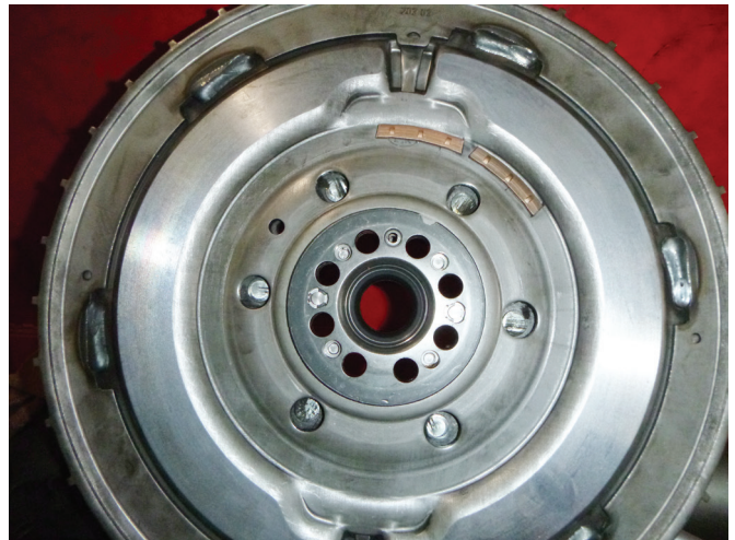
Replacing a flywheel? Pay attention to the clocking. The crank pin goes in the hole at 12 o'clock. If you miss it can behave like a throttle body calibration issue and there is no electrical component test that will guide you to the answer.
