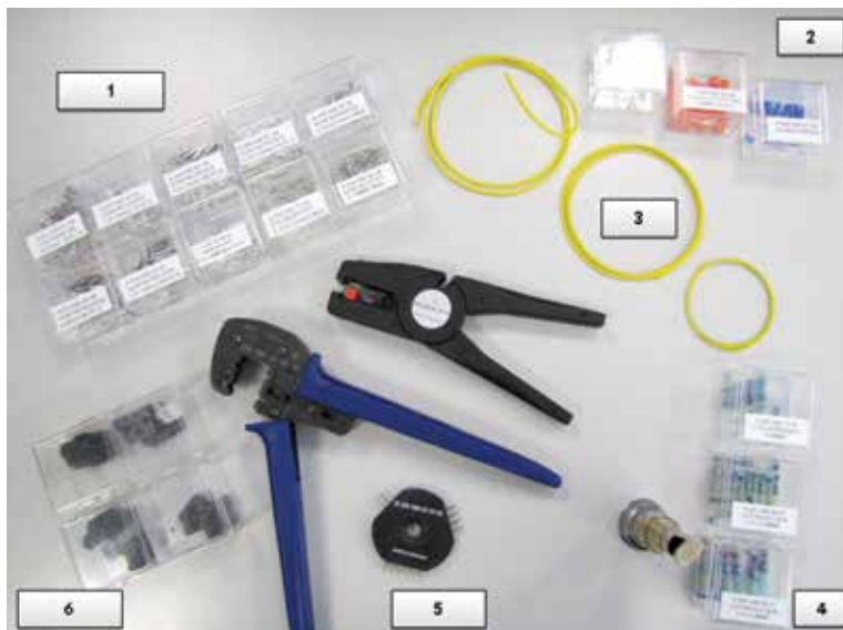
Some of the contents of the Mercedes-Benz wiring repair kit. Contacts (1), seals (2), repair wire (3), Raychem connectors (4), an example of an unpinning tool (5) and crimping pliers with contact-specific die sets (6) are shown, with a wire stripper in the center.
