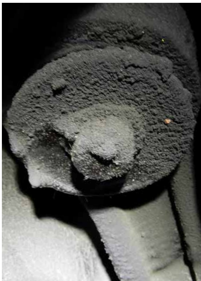
Mounting bolts at differential for viscous coupling
