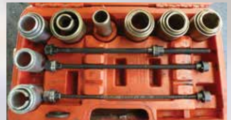
A good bushing press kit can service almost any vehicle that comes into the shop.
