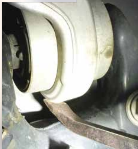
Using light pressure on the bushing with a pry bar can help determine if the bushing has failed.
