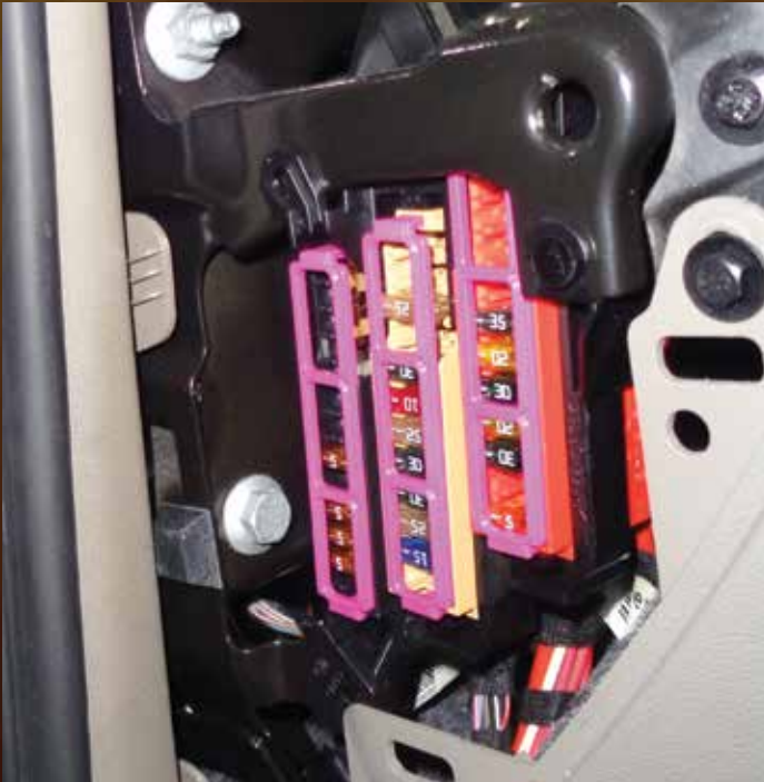
The primary interior fuse block, located at the base of the A-pillar is very susceptible to water damage if there are leaks at the sunroof drains.
