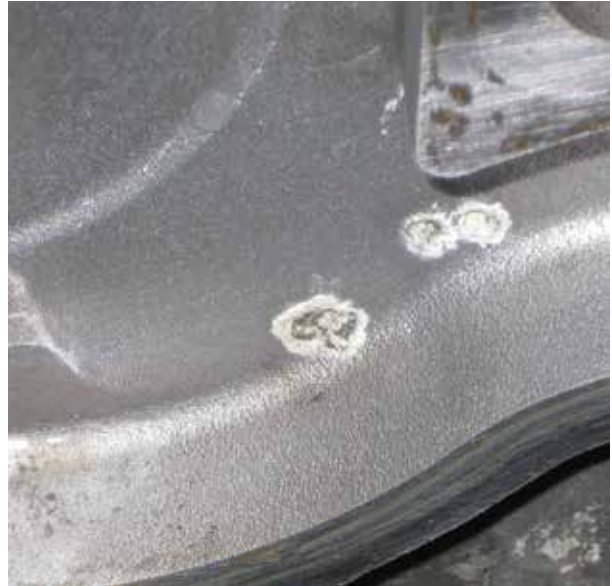
While the corrosion in this water pump housing is just getting started, in a short time it will grow and eventually impede the coolant flow. Genuine Mercedes-Benz antifreeze/anticorrosion protects against this.
