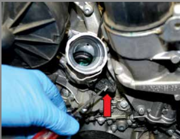
Releasing the electrical connector on the thermostat housing.
