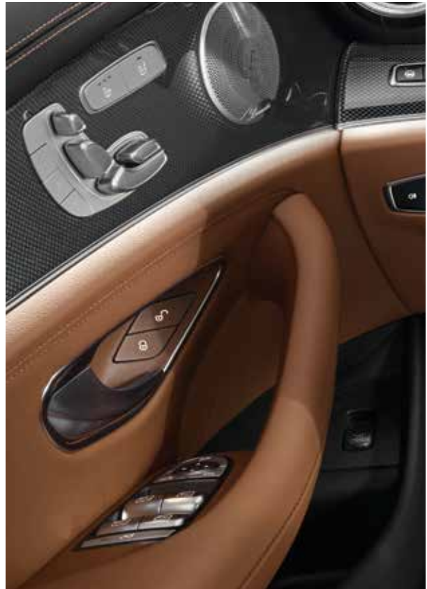
Power window control switches in the door armrest (shown on the 2017 E-Class Sedan) feature one-touch automated or press-and-hold manual operation.
