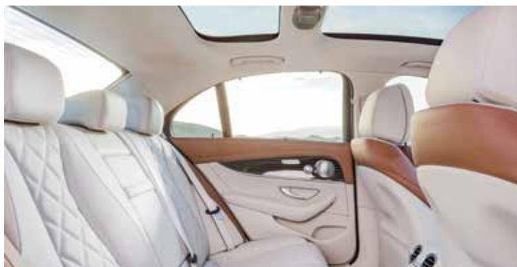
Technicians normalize the side windows, sunroof (shown here on the 2017 E-Class Sedan), and roller blinds (if equipped) by simply pressing and holding the appropriate actuation switch for a short time at its start and end points.
