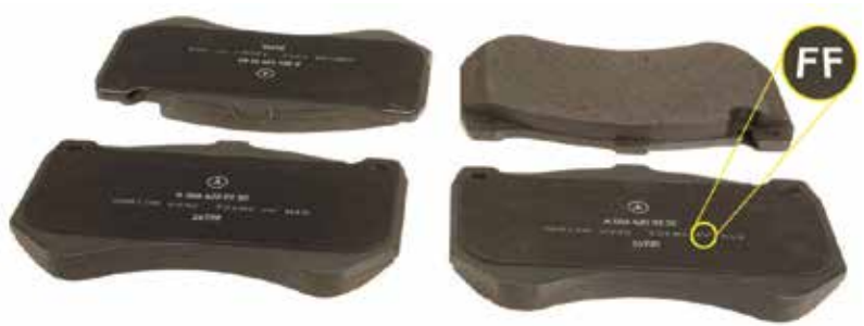
Note the FF designation on these pads for an AMG model
