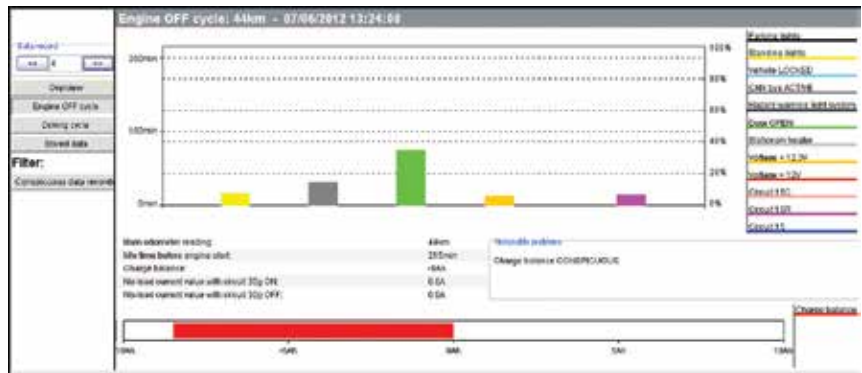
Figure B: An Engine OFF cycle graph. Here, we see that the battery lost about 9 Amp-hours, and several consumers were active, including standing lights and a door that was open for over an hour.
