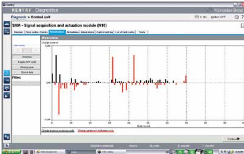
Figure A: The Overview screen shows up to the last 100 driving and engine off cycles, the most recent being #1.
