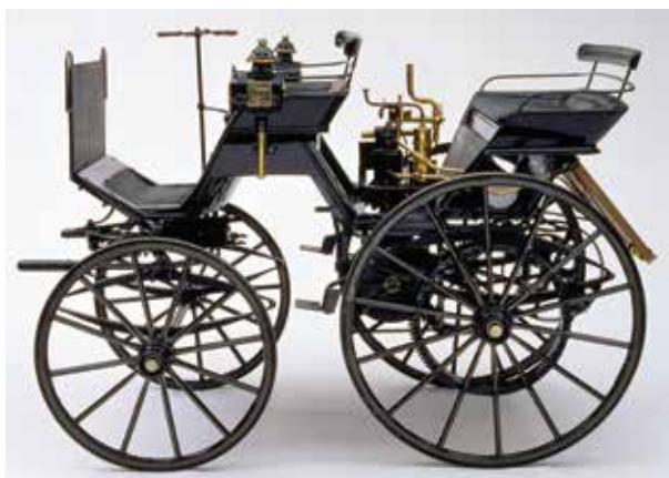
This 1886 model was air-cooled, but went to a water-cooled system in 1887.
