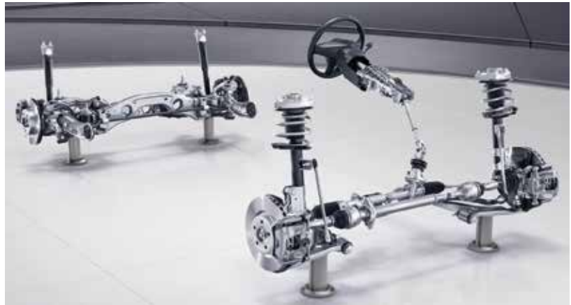
Damage to the adaptive damping system (shown here from the Mercedes-Benz GLA) affects electronic stability control and steering. Pre-scanning narrows the diagnostic path, and post-repair scans help catch additional work, such as steering angle sensor calibration that you must do before delivering the vehicle to the customer.
