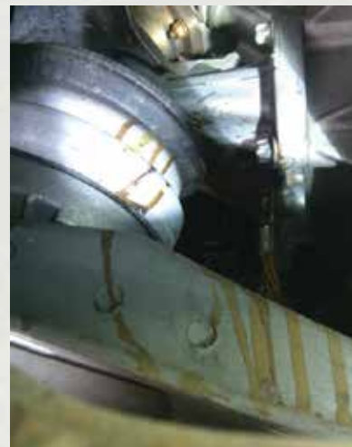
Note the clear signs of a leaking motor mount.
