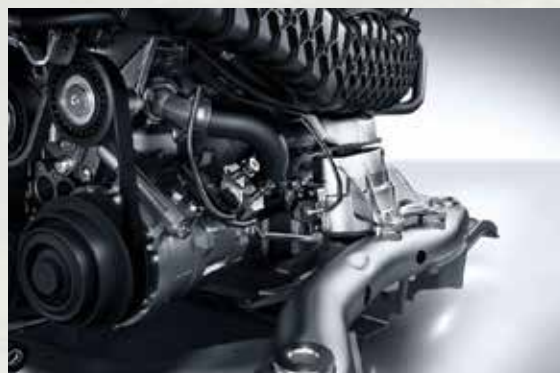
The second-generation MR powertrain mount installed on the AMG C 63 S.
