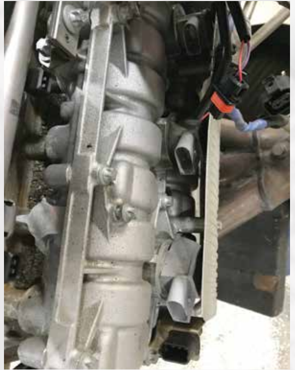
Were it not for the fact that this engine is out of the car, one would not be able to even see these coils. Servicing coils and plugs on this engine requires removal of exhaust components, heat shields and whatever else happens to be in the way.
