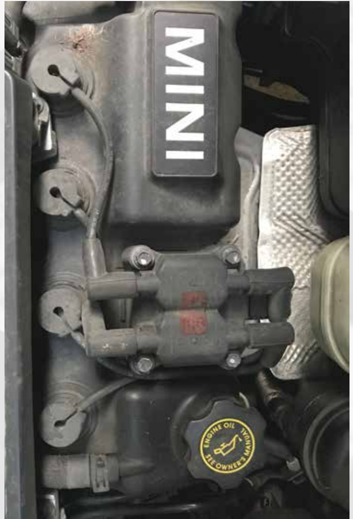
This is a typical waste spark system with one coil firing two cylinders.
