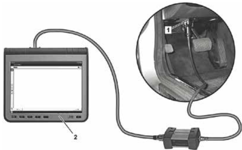
The Mercedes-Benz STAR DIAGNOSIS system allows you to readout factory fault codes that aftermarket scan tools may not be able to access.
