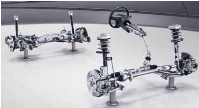
Damage to the adaptive damping system (shown here from the Mercedes-Benz GLA) affects electronic stability control and steering. Pre-scanning narrows the diagnostic path, and post-repair scans help catch additional work, such as steering angle sensor calibration that you must do before delivering the vehicle to the customer.
