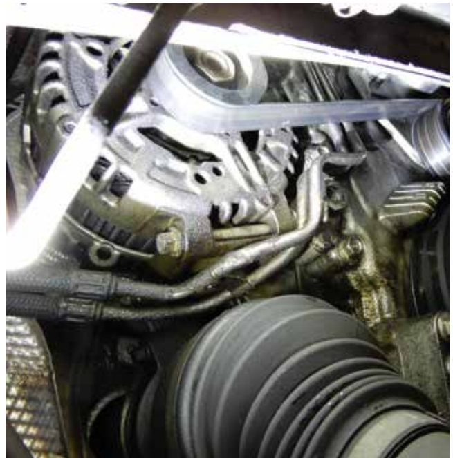
Alternator mounted on engine near firewall
