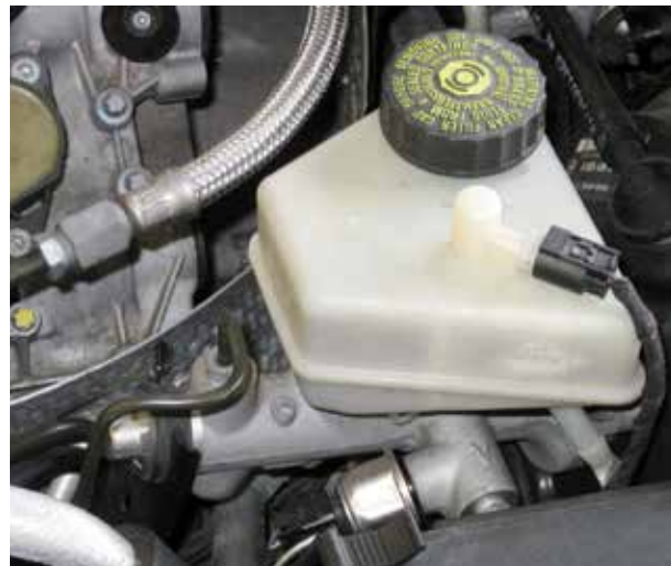
The Brake Operating Unit (BOU) used with SBC looks like a traditional master cylinder, adding a brake pedal position sensor and removing the vacuum booster.
