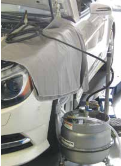
With SBC, a power bleeder and diagnostic scan tool with bleeding routine are an absolute must!
