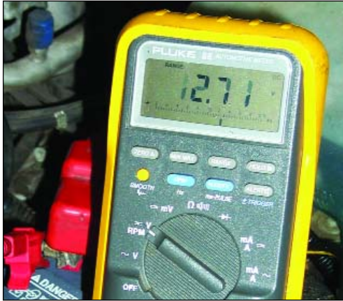
Battery Open Circuit Voltage
