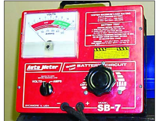
Battery Load Tester
