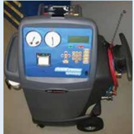
The ROB134APF Air Conditioning Service System with VAS 6337/1A Air Conditioning System Flushing Device offers complete refrigerant recovery, evacuation, recharge and system flushing in a single service machine.
