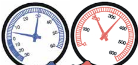
Moisture in system, restrictor ices up
