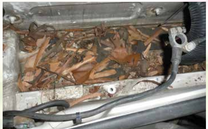
If not periodically cleaned, the cowl area will eventually clog, leading to water ingress.
