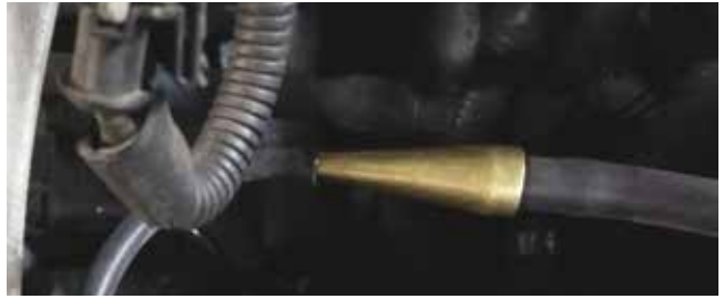
After making a note of the normal parameters, we introduced a small intake vacuum leak and rechecked the data.
