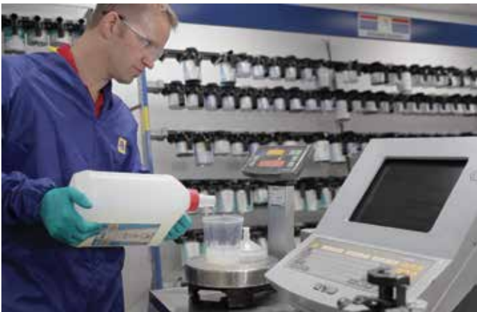
BASF color formula software interfaces with an electronic smart scale to allow pinpoint control of color mixing.
