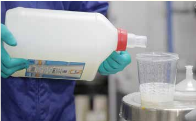
Adding 90-M4EDT (Extended Dry Time) Mixing Clear to Glasurit 90-Line or R-M Onyx basecoats in high heat, low humidity climates prevents paint film from drying too fast for proper pigment flop.
