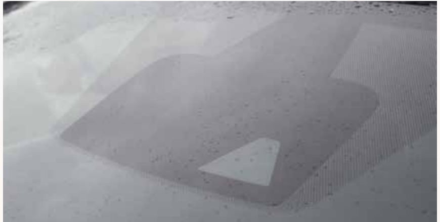
These strange trapezoids in the windshield hide a sophisticated camera that can detect the lane markers on the road and allow the I-LI and LDW systems to help the driver keep the vehicle centered in the lane. Keep in mind, if something affects your visibility, the camera probably can't see either.
