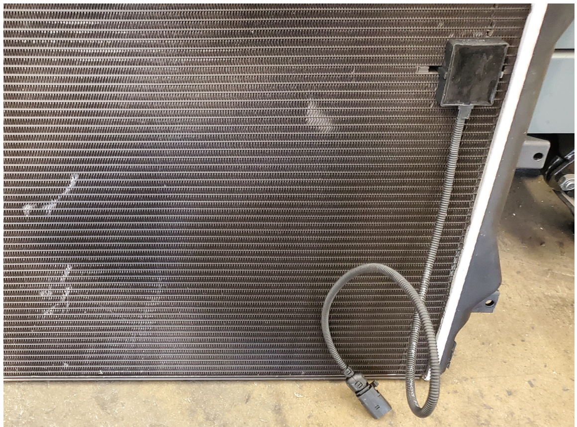
The heat sink area where sensor G611 mounts to the Prem-Air radiator.
