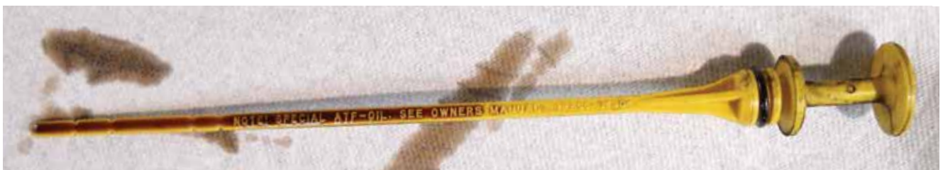
When the transmission fluid is very dark or burnt, you should make sure that the customer understands the possibility of making an already worn transmission worse by changing the fluid. Total transmission failure is rare after a fluid change, but in the event that this should happen you don't want to be left holding the bag.
