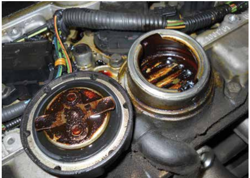
The carbon and oil sludge buildup on this Volvo's oil filler cap is a sure sign that this car has not seen regular service.
