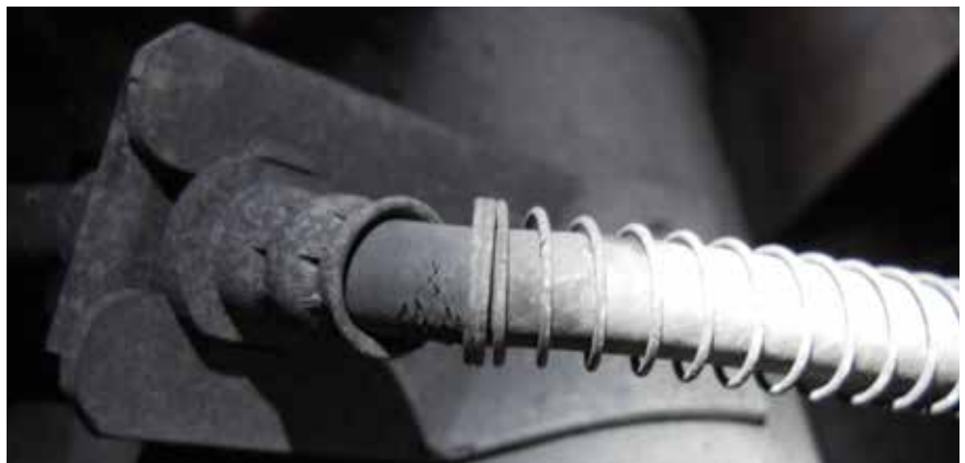
As Volvos and all other makes age, the brake hydraulic hoses will start to develop cracks. If left to continue to deteriorate they can become a serious safety hazard. The hoses for front calipers wear faster than those for the rear because of the constant flexing when the wheels turn.
