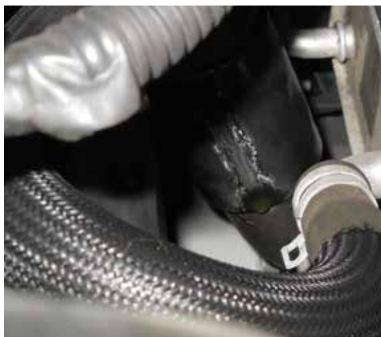
When refilling the coolant on P1 Volvos (2005–present S40/V50/C30/C70) or any Volvos with rubber and bonded plastic radiator hoses, don't use airlift or vacuum filling tools. On older hoses the vacuum can cause the hose to crack and fail prematurely.
