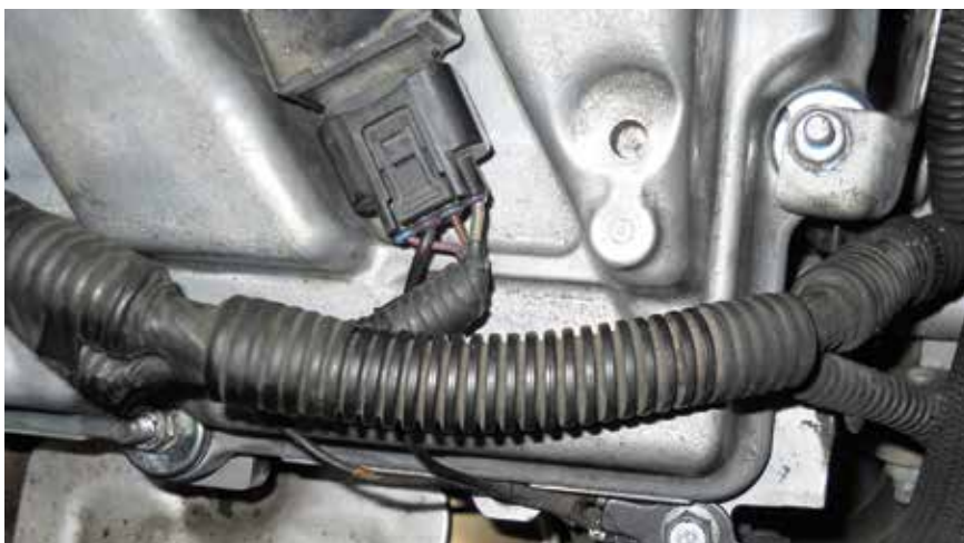
When replacing the valve cover gaskets on Volvo V-8s, take care not to damage the ignition ground wires. They are delicate and can break easily.
