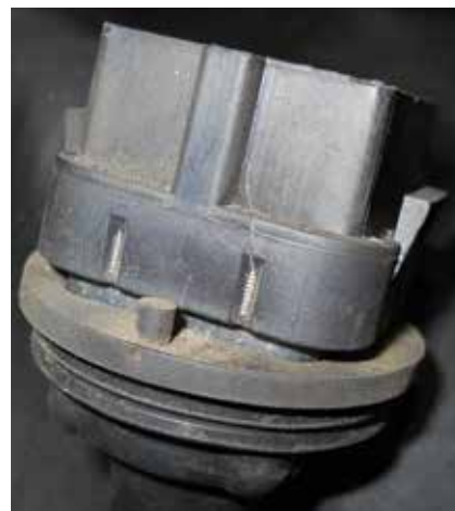
As the coils age they start to develop cracks in the plastic housings, which can let moisture in and leak secondary voltage out.
