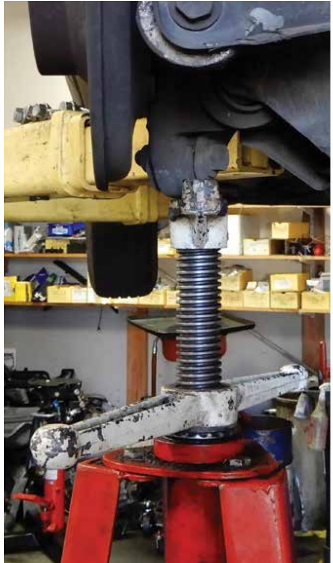
Jack under wheel hub assembly to install lower control arm.
