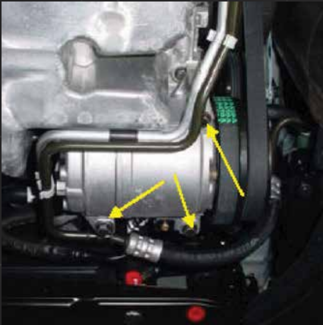
Loosen the 3 bolts on the A/C compressor, 12 mm socket.
