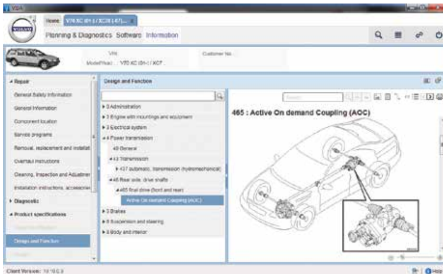
Layout on all wheel drive with Active on Demand (AOD)
