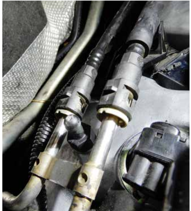
Fuel lines quick disconnect at top of valve cover
