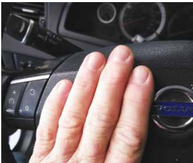
Remove the new SAS sensor's holding screw and install the air bag connectors and press on the air bag.
