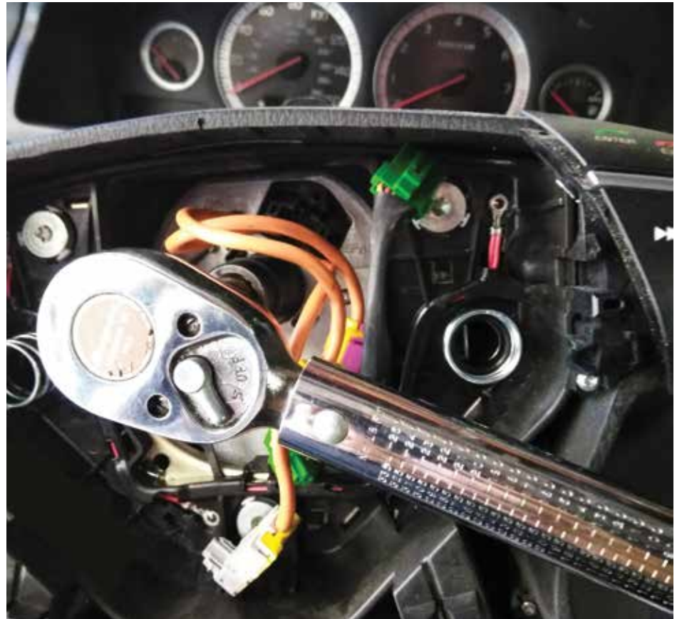
Torque the steering wheel center bolt in two stages: first stage 30 Nm and second stage 30 degree angle torque.
