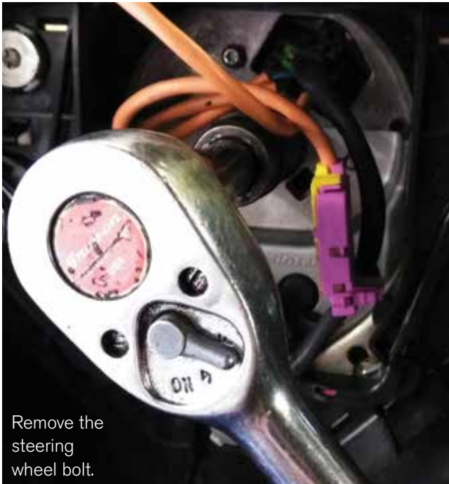
Release the three air bag connectors.
