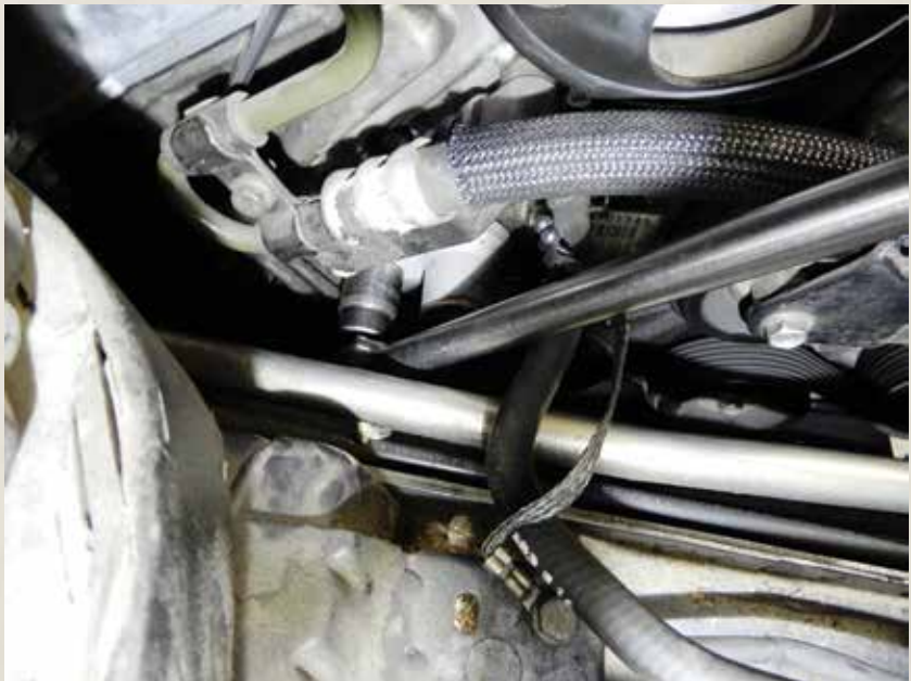
Tool installed to remove pressure on belt tensioner
