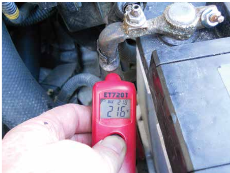
Be careful not to touch the positive clamp during testing on one of these cars, because if the car is running and warmed up, it not uncommon to measure temps over 200 degrees F at the clamp when these cables act up.
