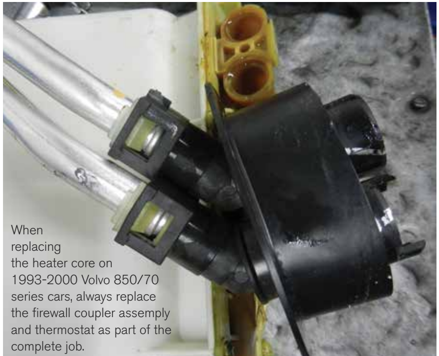
The most common heater core leaks seen at independent shops are those from the 1993-2000 Volvo 850/70 series cars.
