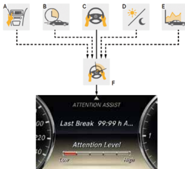
Attention Assist uses several existing sensors and systems to gauge driver fatigue, and issues a warning if actions possibly indicating fatigue are detected.
