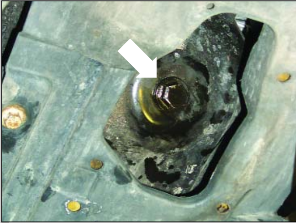
Engine oil drain plug (engine undercover in place)
