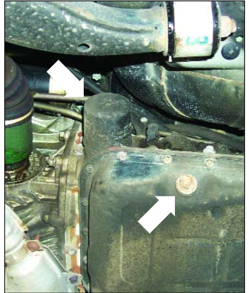
Transmission drain and filter
