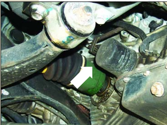
The late model 4EAT has a transmission filter, This filter does not require periodic replacement.
