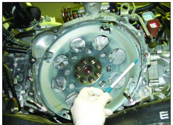
If the transmission must be removed, make sure both dowel pins are in the engine before reinstalling the transmission. Missing dowels will cause alignment problems.
