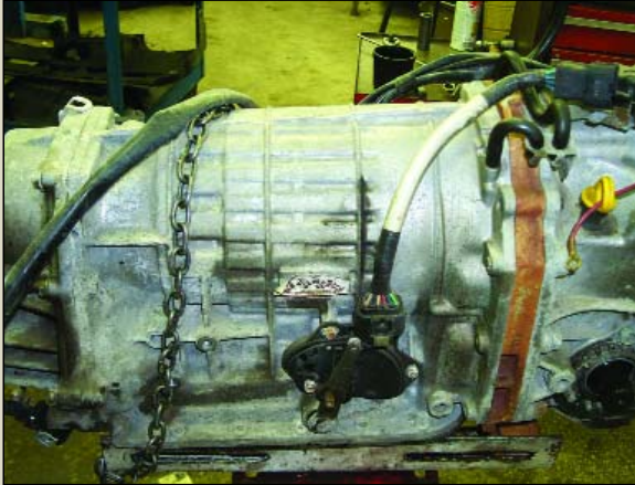
The 2-4 clutch is now splined to the case. Note the external case ribbing.
