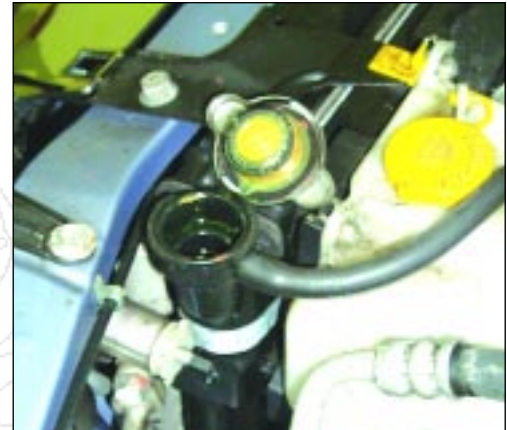
Radiator Cap Inspection
