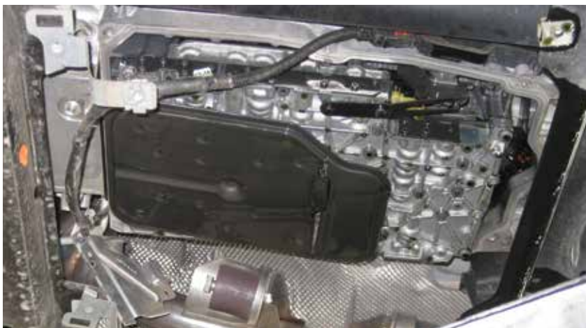
This is the transmission with the oil pan removed. Be sure this area is surgically clean before removing the pan or replacing components.
