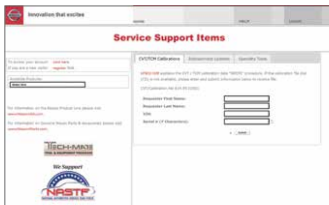
The CVT/TCM Calibrations tab for retrieving calibration file by serial number.
