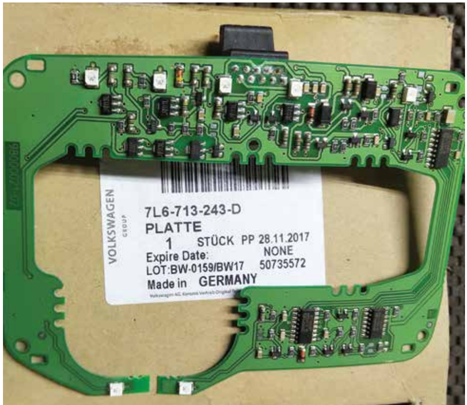
Original circuit board showing the magnetic sensors, from right to left: Park - Reverse - Neutral - Drive - Sport
