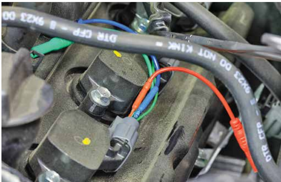
Oscilloscope back probe pins for coil 2
