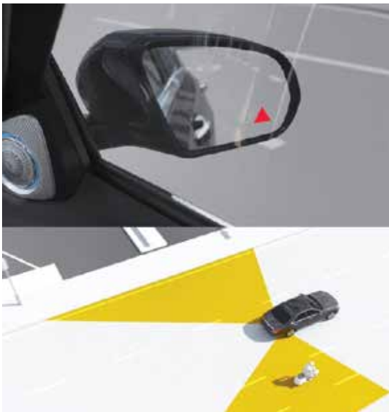
Blind Spot Assist warns the driver of objects detected in the blind spots by lighting a red LED in the mirror.
