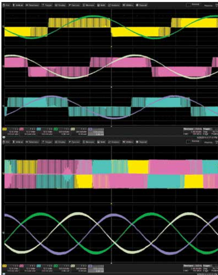
The same 3-phase motor signals, at top shown as voltage/current pairs, and below as voltages (and currents) superimposed. Note how the voltages (yellow, pink, blue) in the lower image seem to vary in amplitude, even though the upper image shows they really do not. Image courtesy Teledyne LeCroy.
