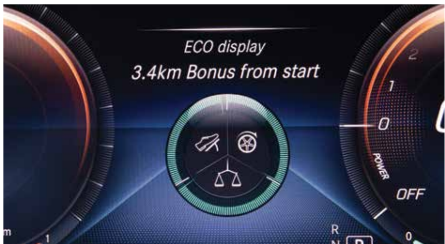
The ECO Display helps inform the driver about power consumption, generation and driving style.
