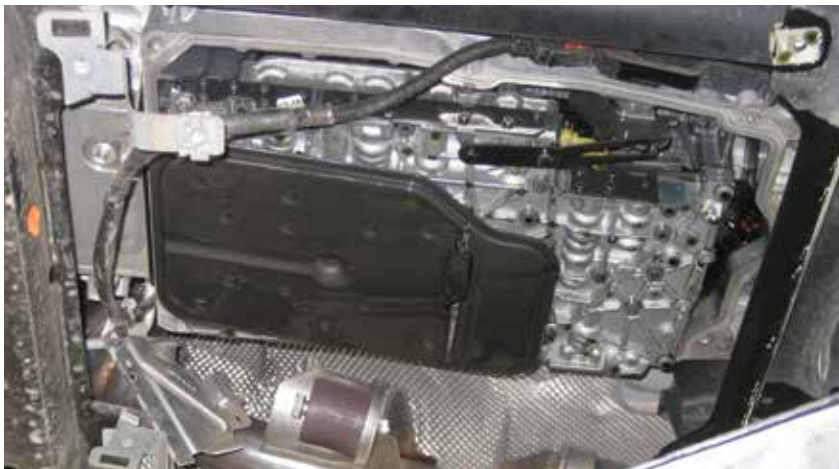
This is the transmission with the oil pan removed. Be sure this area is surgically clean before removing the pan or replacing components.
