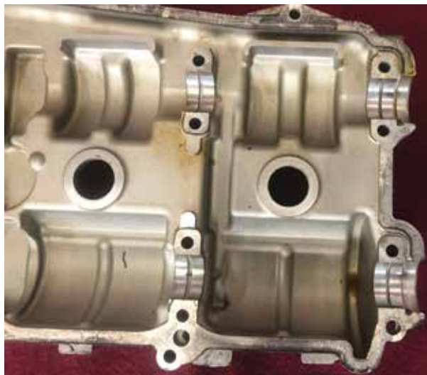
Bearing surfaces: two for the intake cam and two for the exhaust cam are machined directly into the camshaft/valve cover.
