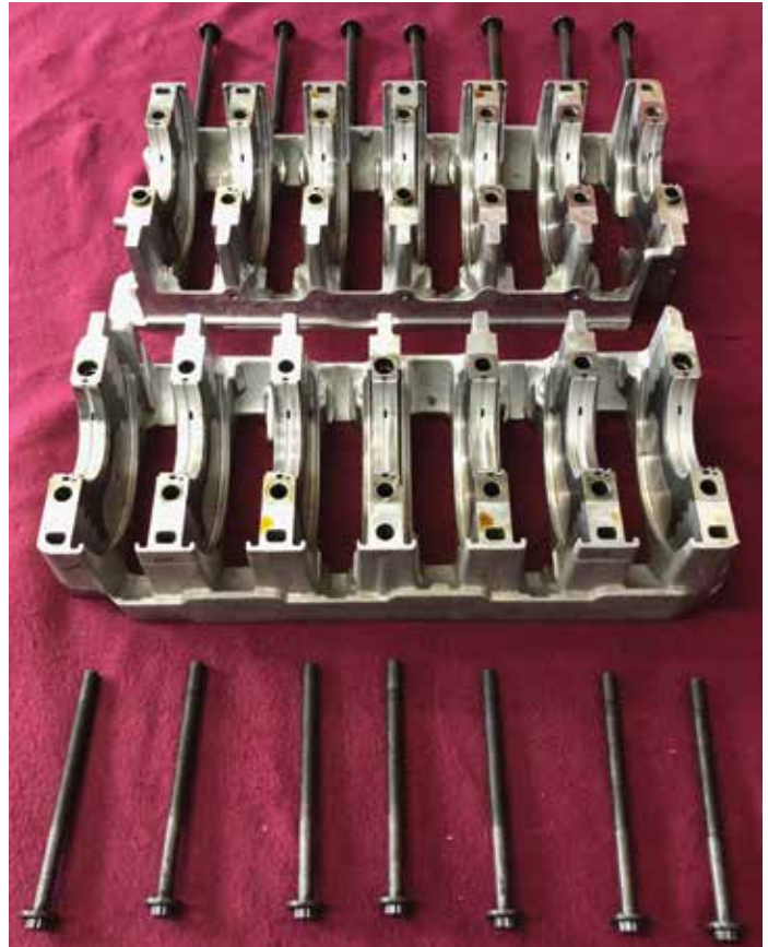
There are a lot of torque-to-yield fasteners in these engines and, as is typical, they all are one time use.
