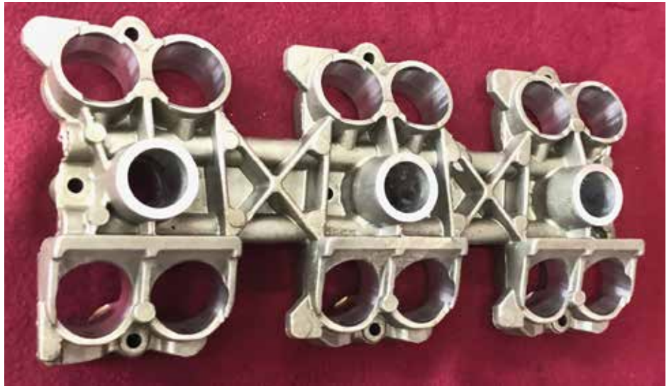
The lifter housing bolts directly to the cylinder head after the camshafts are installed.
