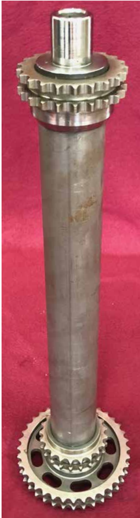
The smaller sprockets at each end drive both cams for each cylinder head. The larger sprocket is driven by a short chain off of the crankshaft.
