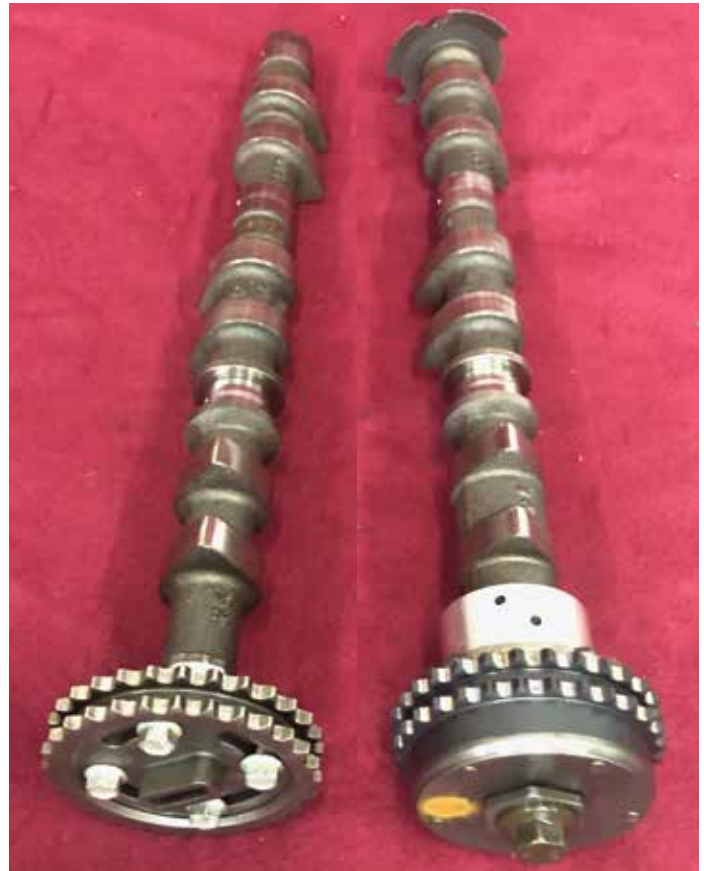
Shown here are the intake and exhaust cams with the timing adjuster on the intake cam and a slotted sprocket on the exhaust cam.
