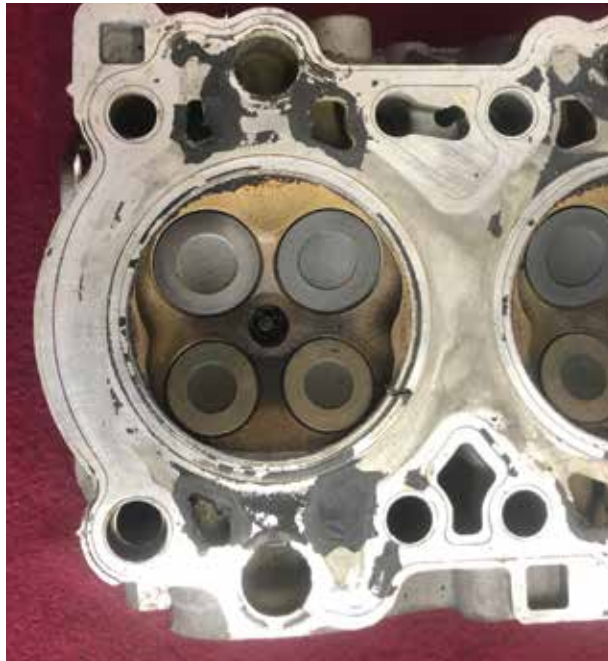
The four-valve design locates the spark plug in the center of the combustion chamber for higher efficiency.
