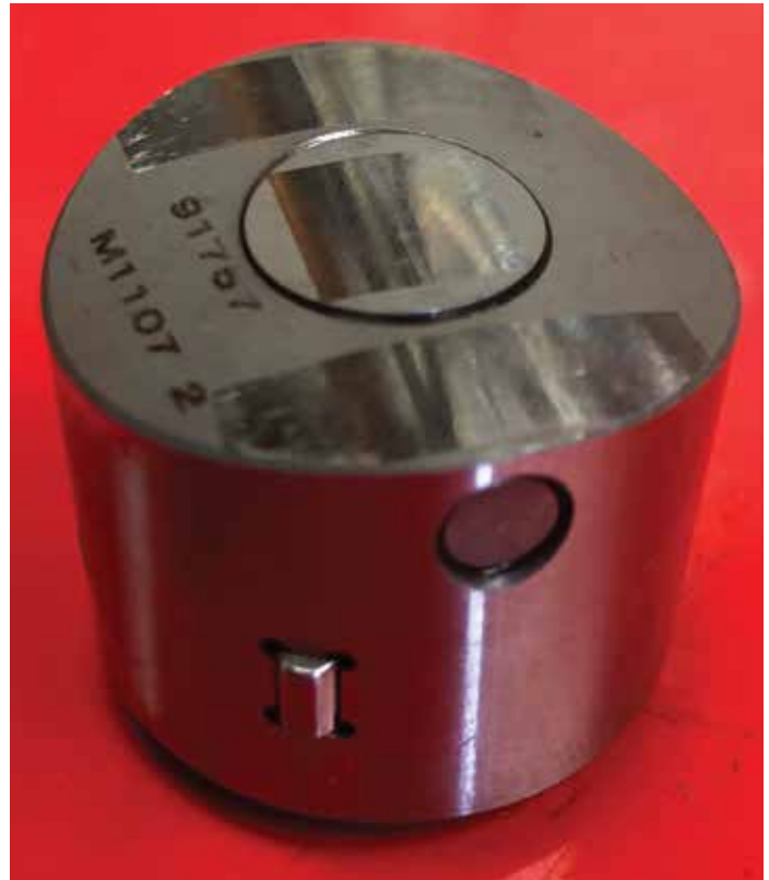
The pin rides in a groove in the bore of the lifter housing.
