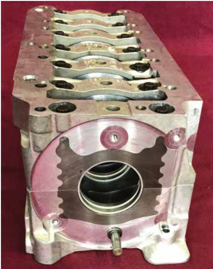
This photo shows the independent crankshaft housing. Steel inserts added strength where it was most needed at the main bearing saddles for the crankshaft.
