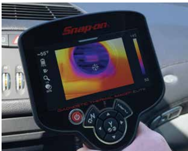
A quality thermal imaging meter can give you accurate duct temperatures.
