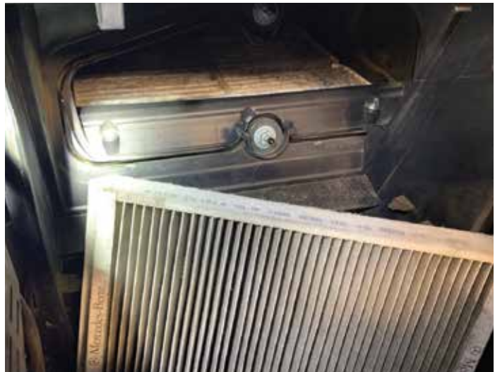
Check those cabin filters! In our shop we've seen even worse than this. Using Genuine Mercedes-Benz filters has many advantages, including superior fit and performance. Consider the StarParts line for price-sensitive customers.
