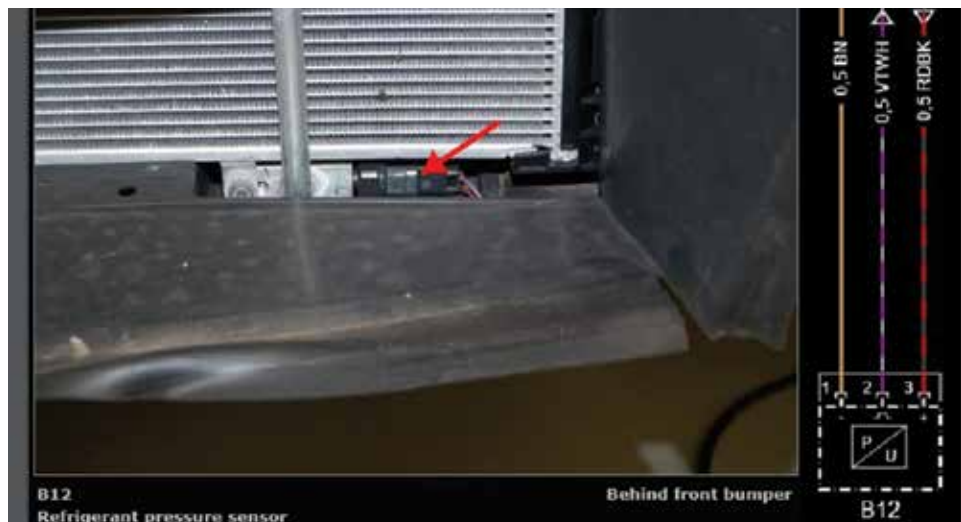
This STAR Finder image shows the refrigerant pressure sensor B12.
