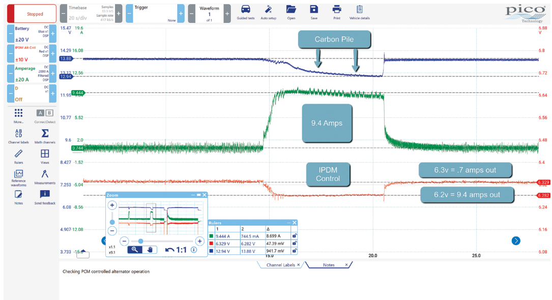
Carbon pile load test - incorrect connections
