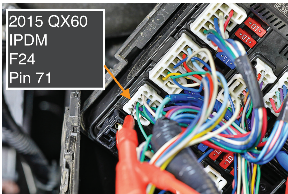
QX60 IPDM alternator control circuit
